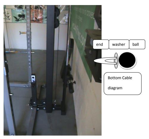
The base cable is similar to the top cable. Make sure the washer is in front of the ball on the cable (see diagram above), if it isn't just slide the ball down the other end of the cable. Secure the cable with an elipse hook.
