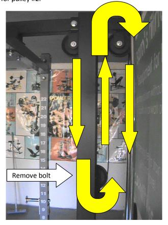
Here you can see the rest of the path for the top cable. You will need to remove a bolt and pulley to get the cable through the two joined pulleys. Run the cable back up to the last top pulley and then bolt the end of the cable into the top of the weight slider unit.
