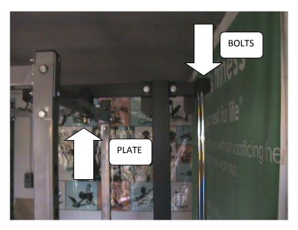
Now bolt the top of the Lat Tower to the rear uprights and rear of the power rack. Don't forget the 2 bolts that secure the chrome slide bars to the top of the Lat Tower. Also remember to have base plate on the underside of the rack
