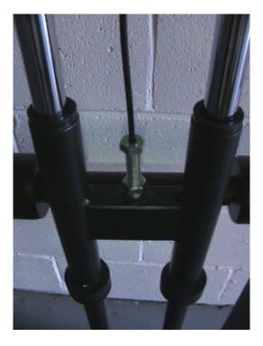
Screw the main bolt down. The nut on the bolt is used to lock the main bolt in place. The bolt pictured is only just in, you will need to screw the bolt in further. Once you have screwed it in you then need to tighten up the lock nut.
