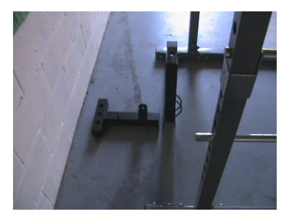
Put the base section of the Lat Tower on the base section of the Power Rack. By lining up the bolt holes you will get it in the right position. Bolt into place, do not tighten any bolts until you have built the entire unit.
