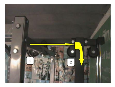
Run the top cable first. The top cable is the one with the bolt at one end. The bolt end screws into the weight slide unit. Run the cable in the direction of the arrows, run the cable through then put pulley #1 in. You will need to run the cable first. Follow the same procedure for pulley #2.
